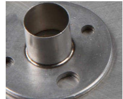
Lasers can be used in many applications including stripping (top) and welding (bottom).
